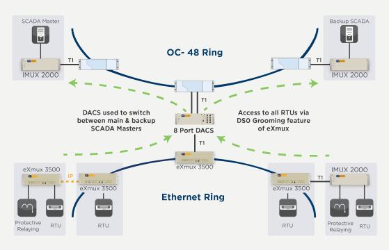
Figure 1: SCADA communications through multi-protocol rings
